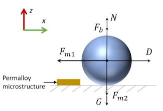
Figure 5. The forces subjected by the single bead captured in the magnetic trap with the micro flow. Flow is in X direction. The bead is displaced downstream of the permalloy microtrap.
