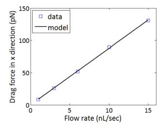
Figure 4. The X component of the fluid-induced drag on the bead in a fully developed micro flow. The relationship between the drag (*D*) and the inlet flow rate (*q*) is described by a linear model ( $R^2$ =0.9995): *D* = 8.786*q*.
