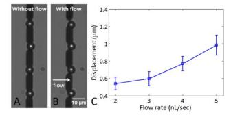
Figure 2. Displacement of single beads in the 3-µm wide traps with the micro flow. Micrograph of beads (A) without and (B) with the flow of PBST at 4 nL/sec. C) The displacement of single beads when PBST was injected at various flow rates.
