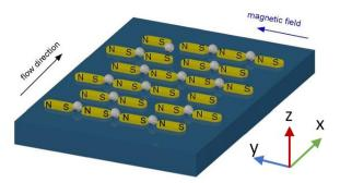
Figure 1. The schematic drawing of single beads trapped by the permalloy microarray on a glass slide. After the introduction of an external magnetic field, permalloy microstructures are magnetized as individual magnets. Single magnetic beads are captured in the gap of two adjacent microstructures.
