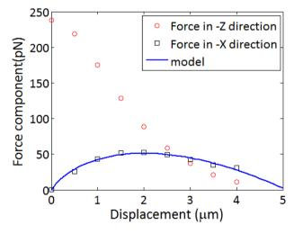
Figure 3. The magnitude of the magnetic force components when the displacement of single beads varied. The relationship between the x component ( $F_{m1}$ ) of the magnetic force and the bead displacement (d) is described by ( $R^2 = 0.98$ ):  $F_{m1} = -150.3d^{1.153} + 192.9d$ .
